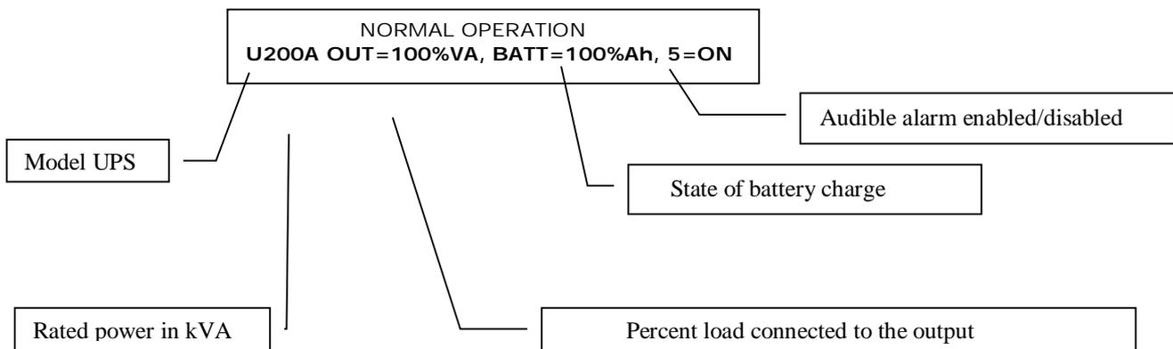
The message U200A indicates an UPS model with 200kVA rated power, operating with 60Hz output frequency. When the unit is set for the parallel operation the letter “P” is added (U200AP). The letter “P” became lower case “p” when the unit operate as slave.
