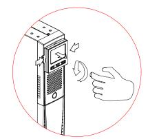
2 - Rotate the panel 90° counter clockwise and reinsert it carefully into the special housing.
