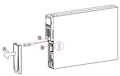
3. Remove the battery pack's retention panel carrying out the operations shown in the figure below.
