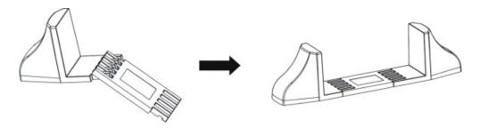
Slide the UPS and the battery box into the two supports
