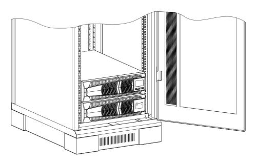
Example of UPS and BATTERY BOX installed in a rack cabinet
