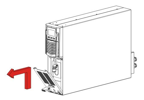
4. Slip off the battery pack pulling it towards the outside, as shown in the figure below. Be careful when extracting and lifting up the battery pack as it is heavy. ATTENTION: the new battery pack must contain the same number and type of batteries (see the label located on the
