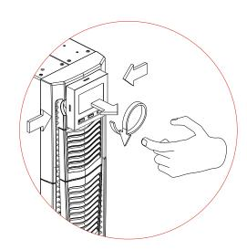
3. At this point, with the UPS or Battery Box in the horizontal position, secure the handles using the screws provided, as shown in the figure.
