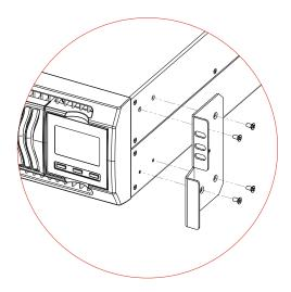
**NOTE:** Given the heavy weight, the use of support brackets is mandatory during rack installation (guide with L-shaped support). For the same reason, it is recommended that the UPS and Battery Box be installed in the lower part of the rack cabinet.
