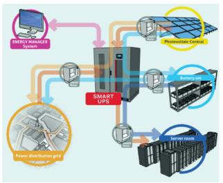
For example, during peak offer periods (at night) and when the energy cost is lower, it is possible to create an energy reserve of the STORAGE device to be used during peak demand periods (during the day) when the energy cost is higher, or to ensure peak shaving and avoid costly increases in the contractual power or penalties for exceeding the maximum power thresholds.
